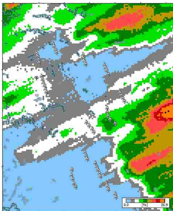
Figure 27 - Turbine sites where WASP underestimates production by 10% and over, mapped with RIX grid and surface roughness polygons. Figure shows maps of prevailing wind direction (bottom) and wind directions for section 30° to either side (Top).
